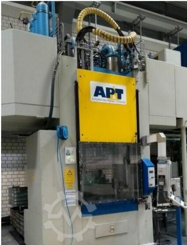
Presskraft 4000 kN
